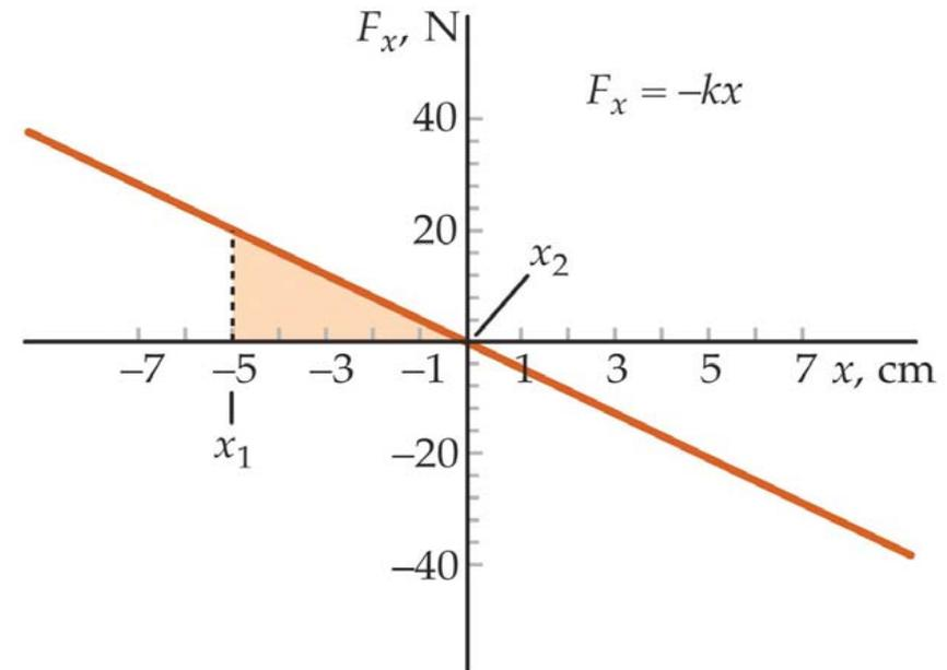
$$\text{aus } W = \int_{x_1}^{x_2} F_x dx \quad \text{mit } F_x = -kx \Rightarrow$$
