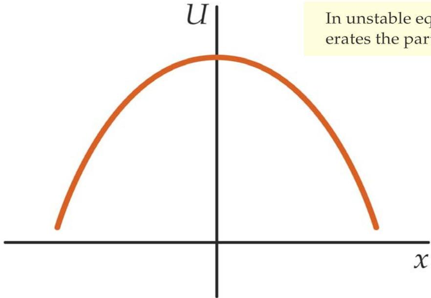
In unstable equilibrium, a small displacement results in a force that accelerates the particle away from its equilibrium position.
