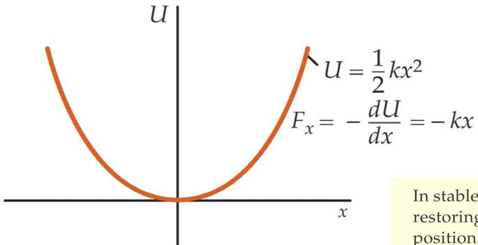
In stable equilibrium, a small displacement in any direction results in a restoring force that accelerates the particle back toward its equilibrium position.
